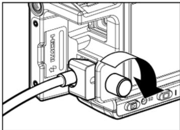
HU-11 comes with an HDMI cable lock that prevents the HDMI cable from being disconnected when shooting images.
