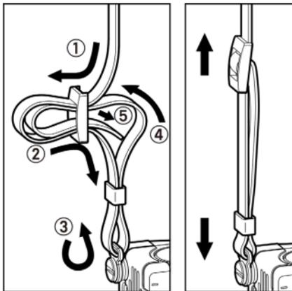
Undo both ends of the supplied strap and attach it to the right and left strap holders as shown.
