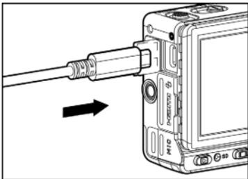
If the USB port of your PC is type C, connect your SIGMA fp L to your PC using the USB cable provided with the camera. If the port is type A, connect your SIGMA fp L using a commercially available USB cable (A to C).
