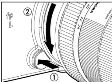
To remove the lens, press the lens lock button and turn the lens counter-clockwise until it stops. Gently remove the lens from the camera body.
