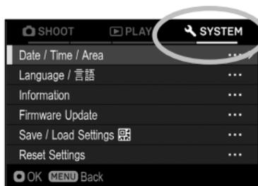
When the camera is being used for the first time or if it has not been used for a long time, set the correct date, time, and area.
