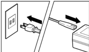
You can power the camera from a wall outlet using the AC adapter set SAC-7P (sold separately).
