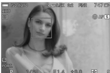
When a face and an eye are detected, the orange detection frame is displayed.
